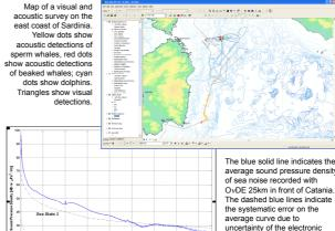
average sound pressure density of sea noise recorded with OvDE 25km in front of Catania. The dashed blue lines indicate the systematic error on the average curve due to uncertainty of the electronic noise power spectrum. The black curves indicate respectively the expected SPD of the sea in conditions of Sea State 0 and Sea State 2.
