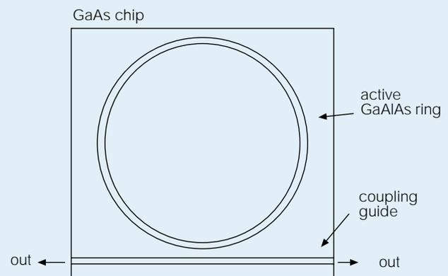
Figure 1 Ring laser schematics.
