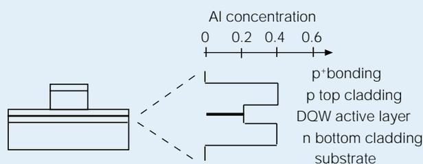
Figure 2 Waveguide details.
