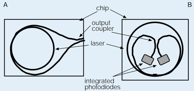
Figure 3 Output coupler options. A off-chip output; B with integral photodiodes.
