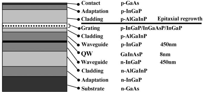
Fig. 1. Vertical laser structure.
