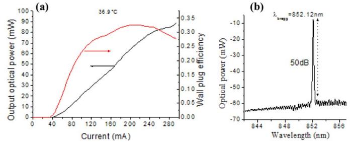
Fig. 3. (a)  $L$ – $I$  and plug efficiency characteristics of 2-mm-long uncoated DFB laser diode at 36.9 °C. (b) Spectral characteristics of the DFB 2-mm-long laser at 852.12 nm and  $T = 36.9^\circ\text{C}$ .
