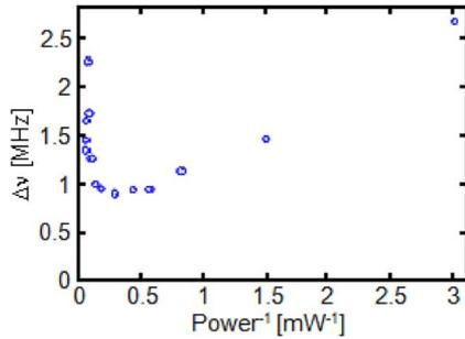
Fig. 4. Variation of measured linewidth with respect to the inverse of optical power.
