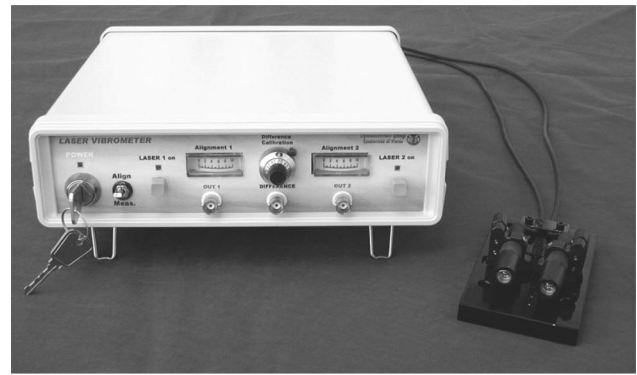
Fig. 7. Picture of the assembled differential vibrometer.
