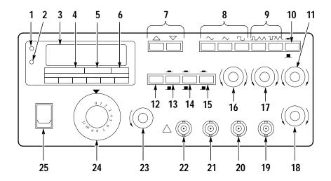
Figure 2: Front Panel Controls, Connectors, and Indicators
