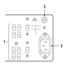
Figure 1: Line Voltage Selectors, Power Input, and Fuse Locations
