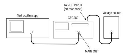
Figure 6: External Sweep Test Setup
