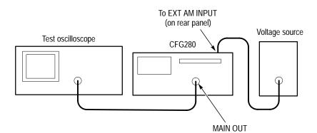
Figure 7: Amplitude Modulation Test Setup
