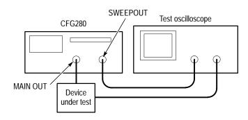
Figure 5: Internal Sweep Test Setup
