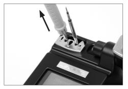
Pull slightly to remove the cartridge
