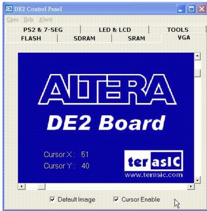
Figure 11.13 Display default image and use the scrolling bars to control cursor moving
