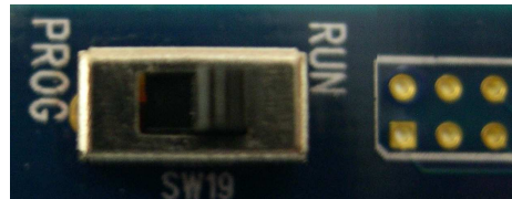
Figure 5.4. Switch Position should be kept at RUN for JTAG/Normal Operation
