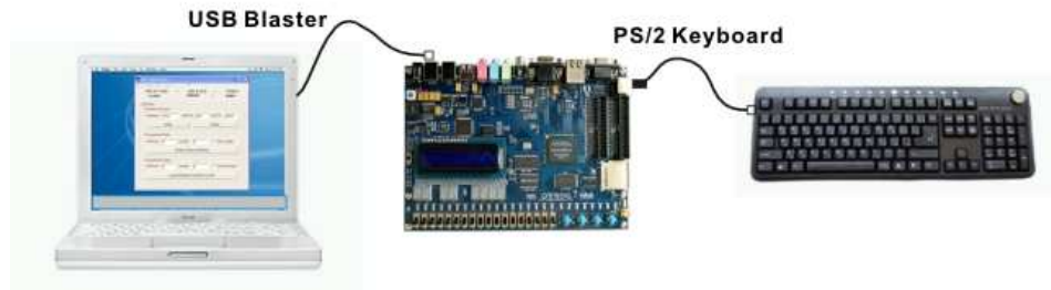
Figure 11.9 PS2 and USB/RS232 connection Setup
