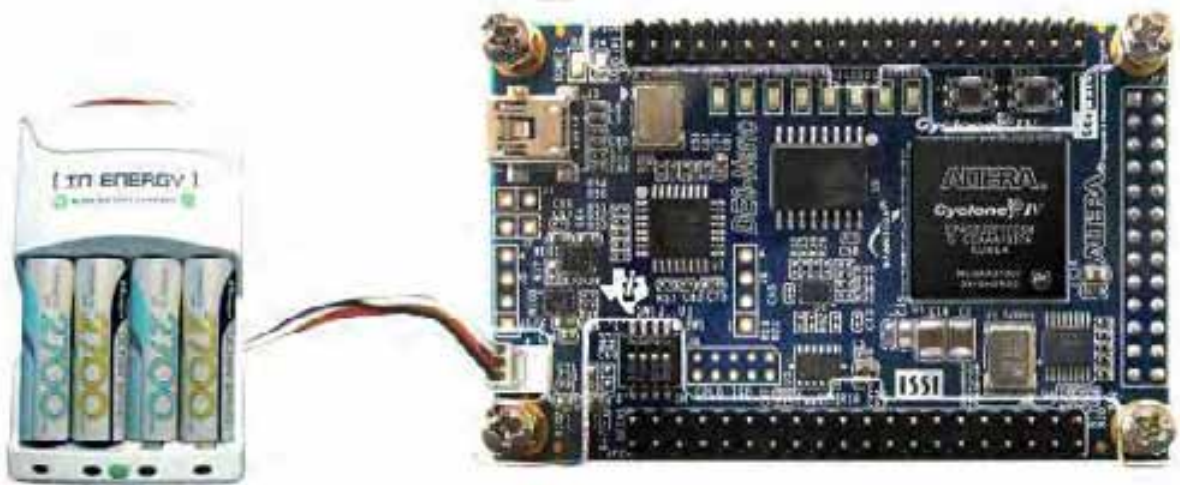
Figure 3-15 Portable Battery Connection
