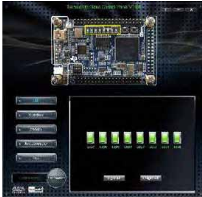
Figure 4-1 The DE0-Nano Control Panel
