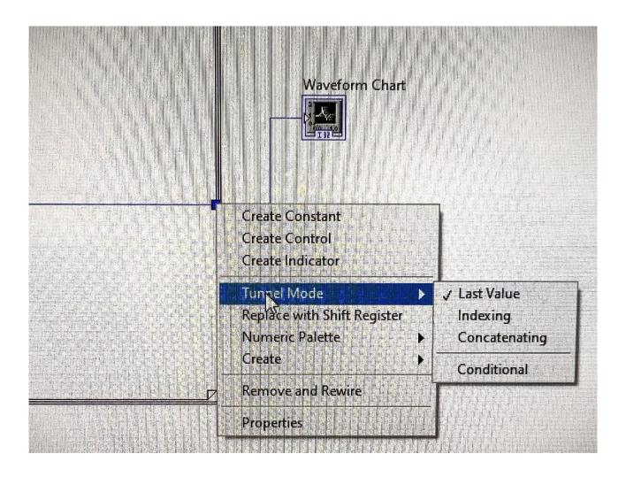
Until LabView 2020 (before latest auto-updates), the default option for coming out from cycles with a signal was that such signal, if scalar, was the last value in the loop complete execution.
