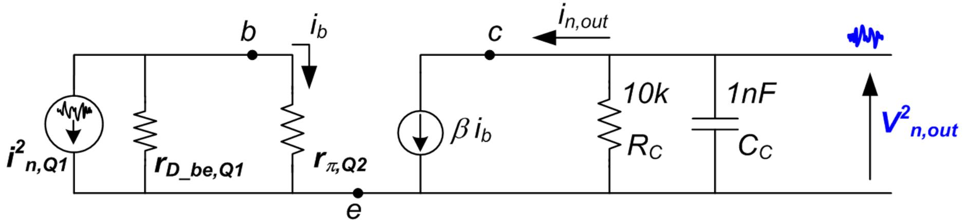
$$i_{n,out}^2 = \hat{i}_{n,Q1}^2 \frac{r_{D\_be,Q1}}{r_{D\_be,Q1} + r_{\pi,Q2}} \quad [A^2 / Hz]$$
