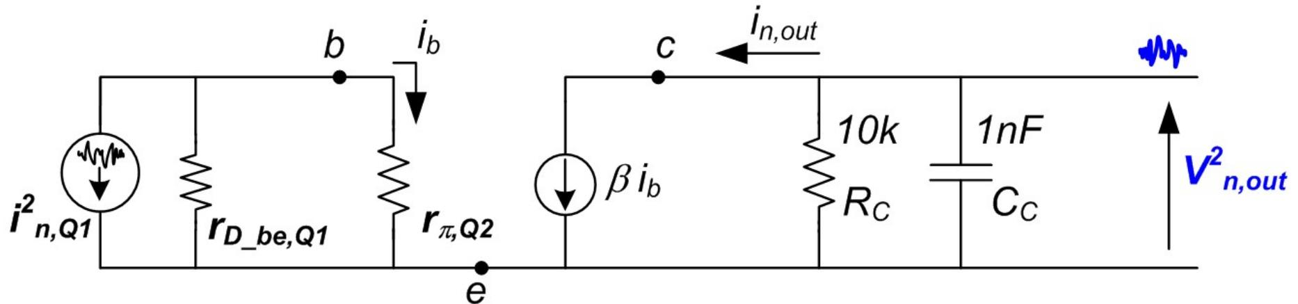
$$i_{n,out}^2 = \left[ i_{n,Q1} \left( \frac{r_{D\_be,Q1}}{r_{D\_be,Q1} + r_{\pi,Q2}} \right) \cdot \beta \right]^2 \quad [A^2 / Hz]$$
