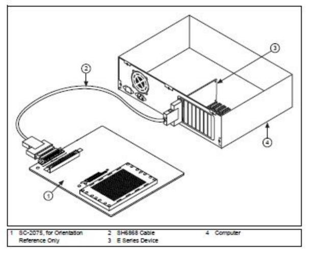
The breadboard is connected to the DAQ board through an 80 pin flat cable
