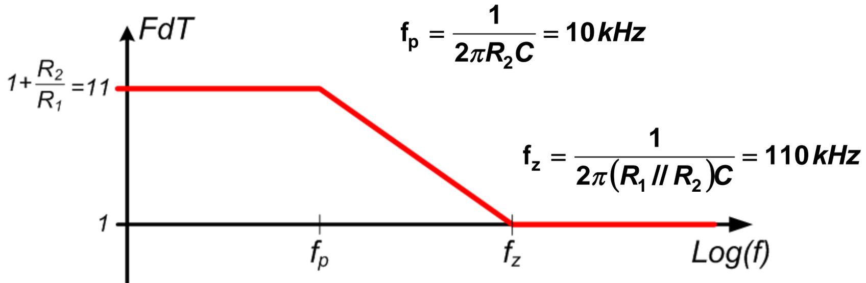
$$f_p = \frac{1}{2\pi R_2 C} = 10 \text{ kHz}$$
