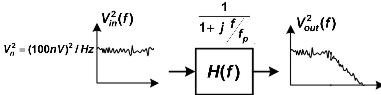
$$V_{out}^2(f) = V_{in}^2(f) \left| \frac{1}{1 + j f / f_p} \right|^2 = V_n^2 \frac{1}{1 + \left( \frac{f}{f_p} \right)^2}$$
