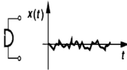
$$P = \lim_{T \rightarrow \infty} \frac{1}{T} \int_0^T \frac{X^2(t)}{R_L} dt \quad [\text{Watt}]$$
