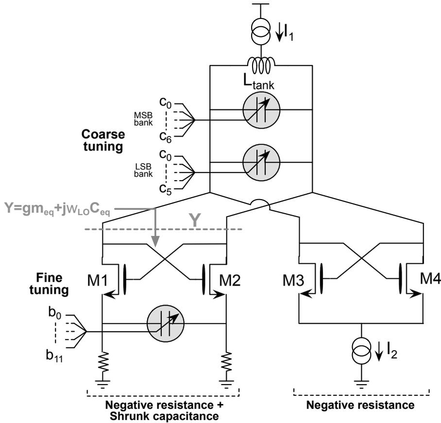
Figure 2.6: ADPLL digitally controlled oscillator scheme
