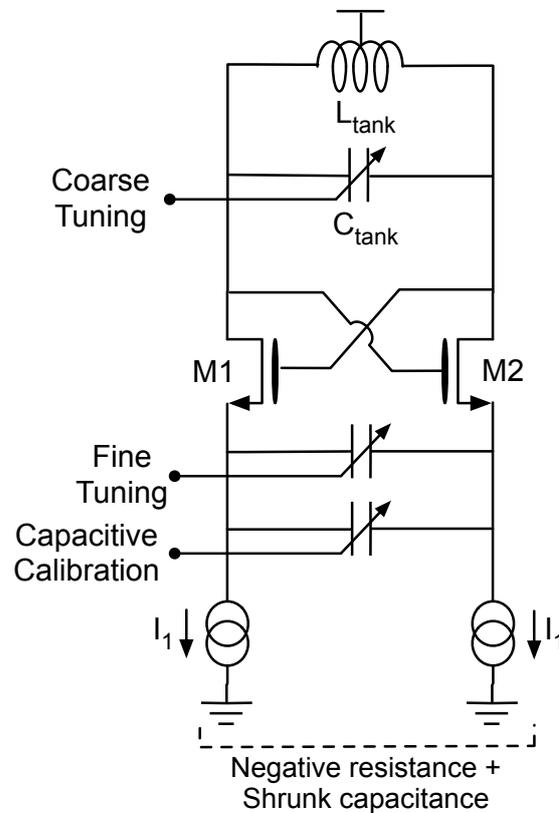
**Figure 1.12:** Capacitive calibration of the DCO capacitive degeneration.
