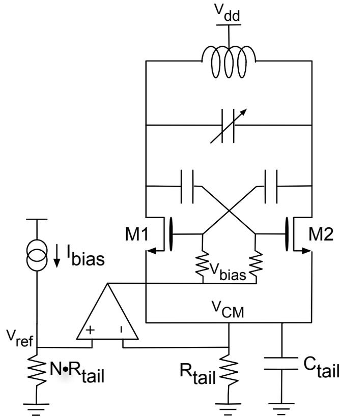
**Figure 3.8:** Schematic of the proposed class-C VCO with tail resistor
