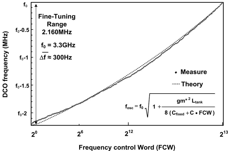
**Figure 4.5:** *Fine-Tuning characteristic*
