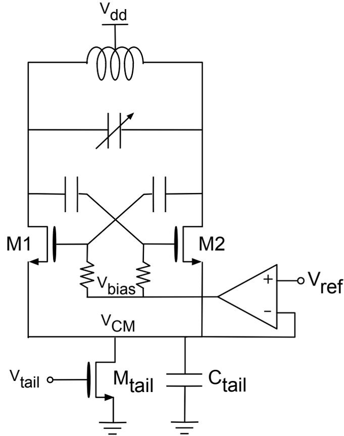
**Figure 3.6:** Schematic of the proposed class-C VCO with current generator
