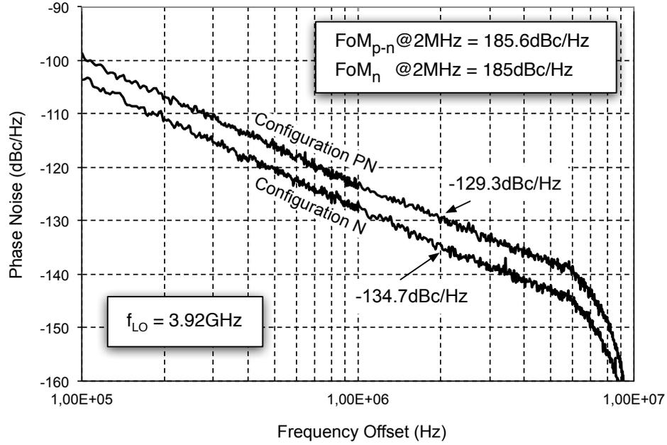
**Figure 4.17:** Phase noise measurements of the two DCO configurations
