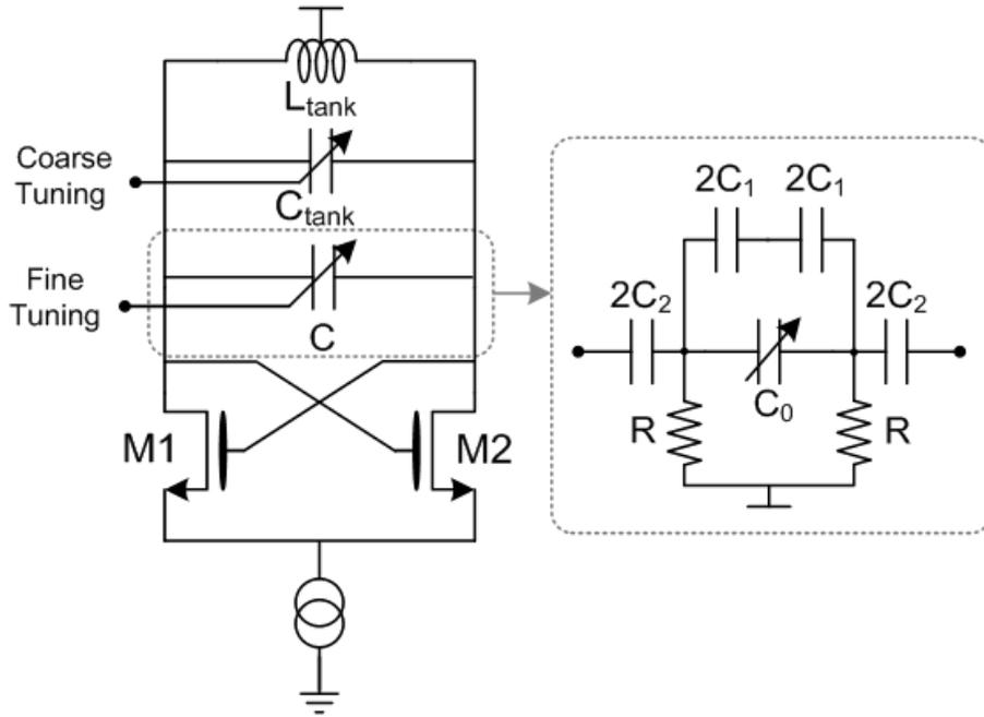
Figure 1.4: Scheme of the capacitive divider network.
