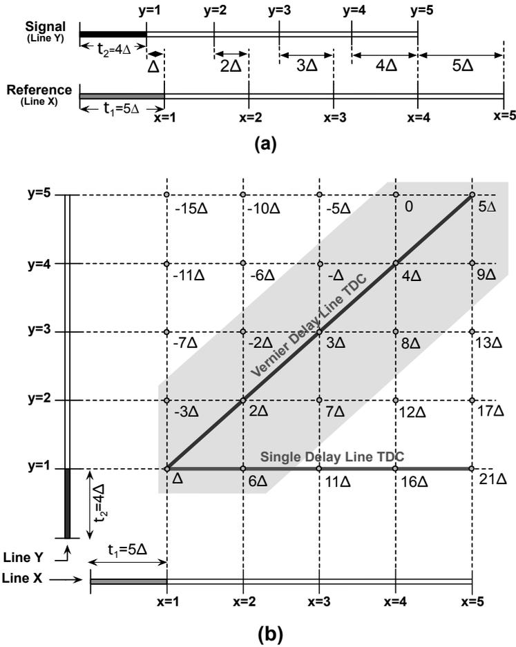
Figure 2.2: (a) linear and (b) 2-dimension Vernier TDCs.
