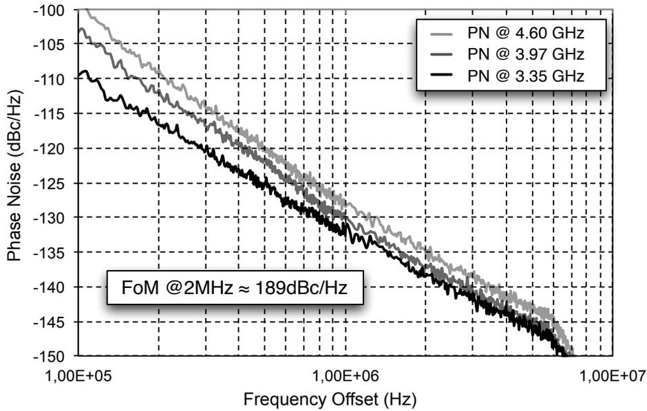
**Figure 4.20:** Phase noise measurements at the minimum, middle, and maximum oscillation frequency
