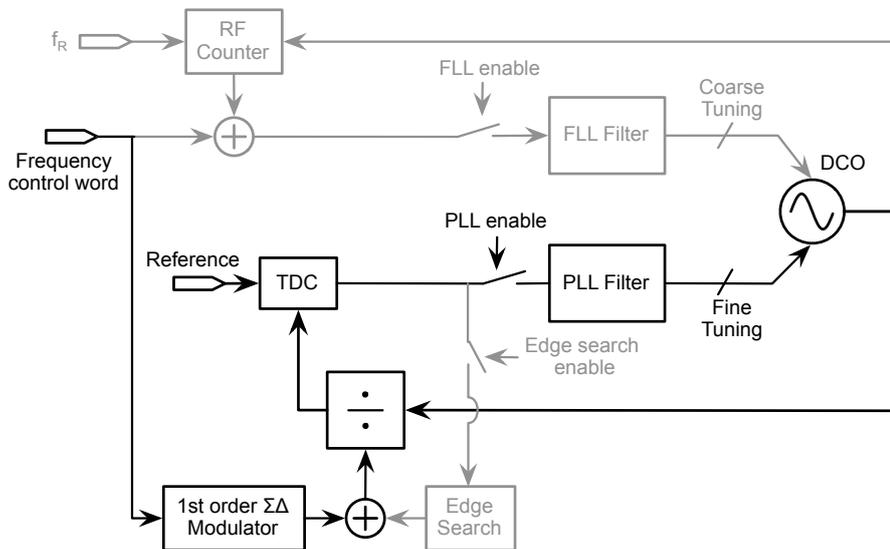
Figure 2.12: Phase locking and Gear Shift
