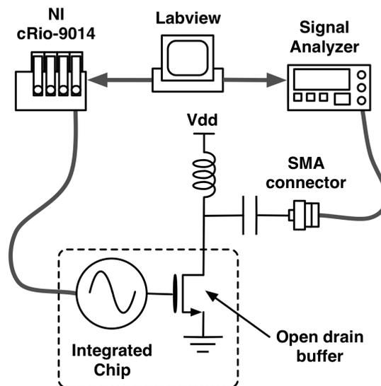
**Figure 4.4:** Environment setup
