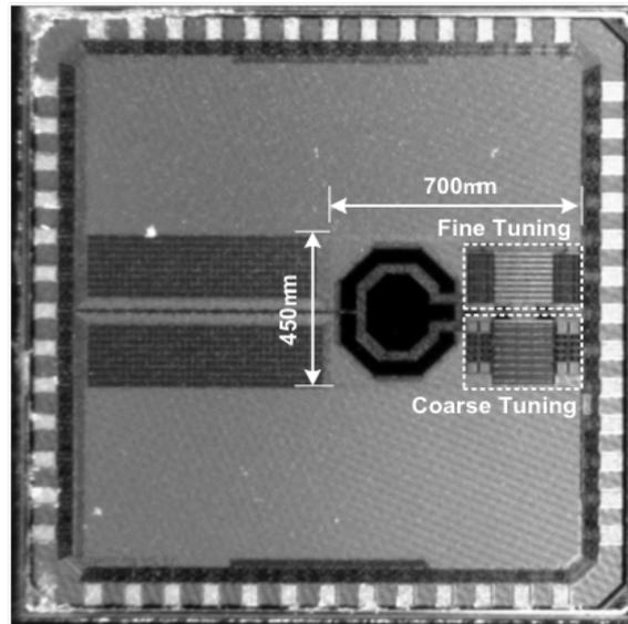
**Figure 4.3:** Chip Photograph of the DCO.
