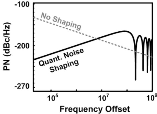
**Figure 1.6:** Phase Noise comparison between dither and dither-less solutions.
