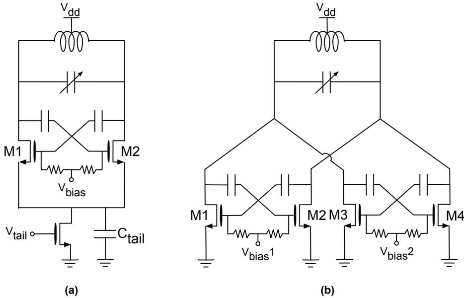
**Figure 3.4:** Original class-C oscillator [17]; b) dual-conduction oscillator [35]
