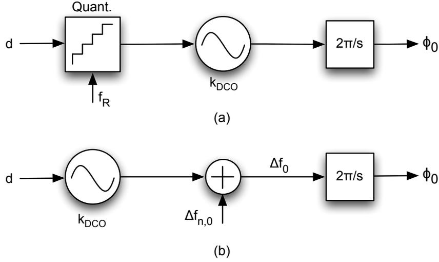
**Figure 1.2:** Model of the quantization noise of the DCO.
