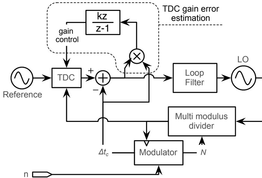
**Figure 2.4:** TDC gain calibration loop
