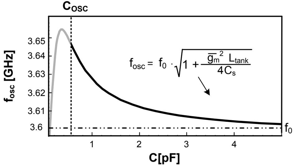
**Figure 1.10:** DCO fine frequency tuning ( $g_m = 10mS$ ).
