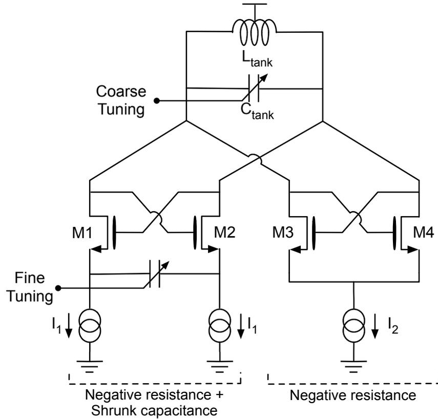
**Figure 1.11:** Current calibration of the DCO capacitive degeneration.
