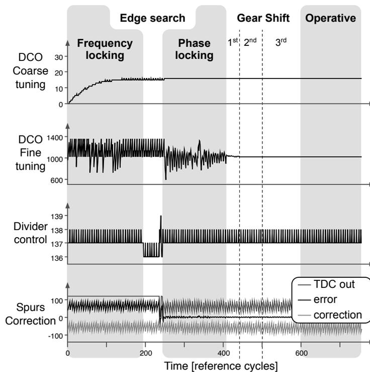
Figure 2.13: ADPLL locking procedure simulation
