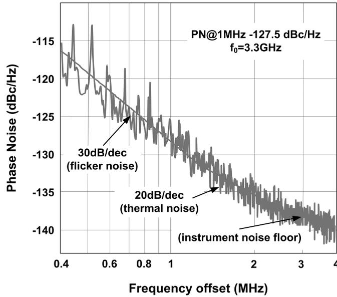
Figure 4.7: Output phase-noise measure
