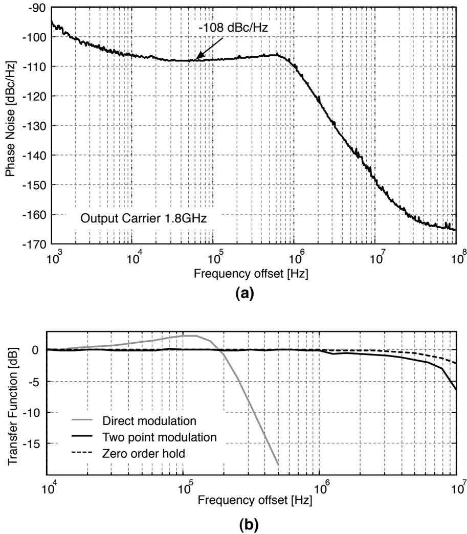
**Figure 4.13:** (a) Phase noise and (b) PLL transfer function
