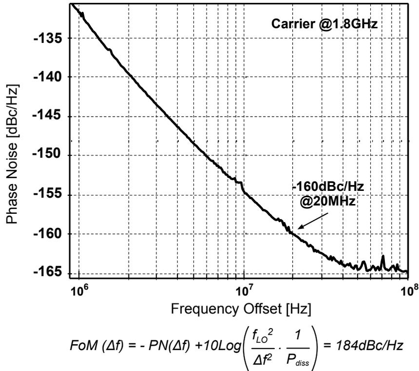
**Figure 4.10:** Phase noise open loop DCO
