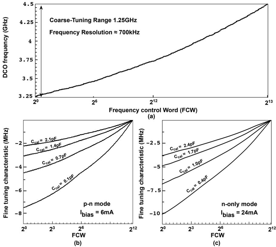
**Figure 4.16:** (a) Coarse tuning characteristic. Fine tuning characteristics for p-n mode (b) and only-n mode (c)
