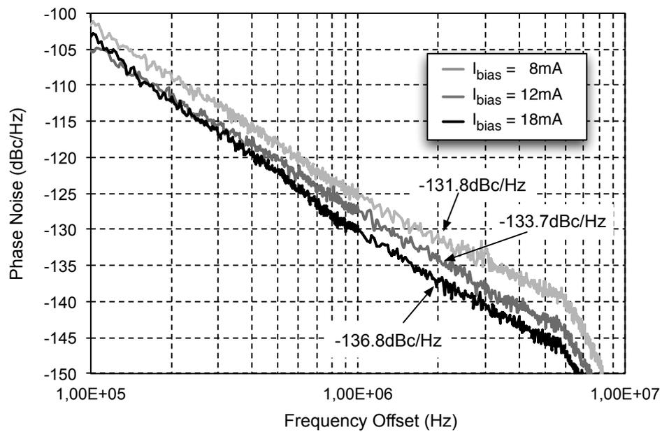
**Figure 4.24:** Phase noise measurements at mid-band, for different values of bias current  $I_{bias}$
