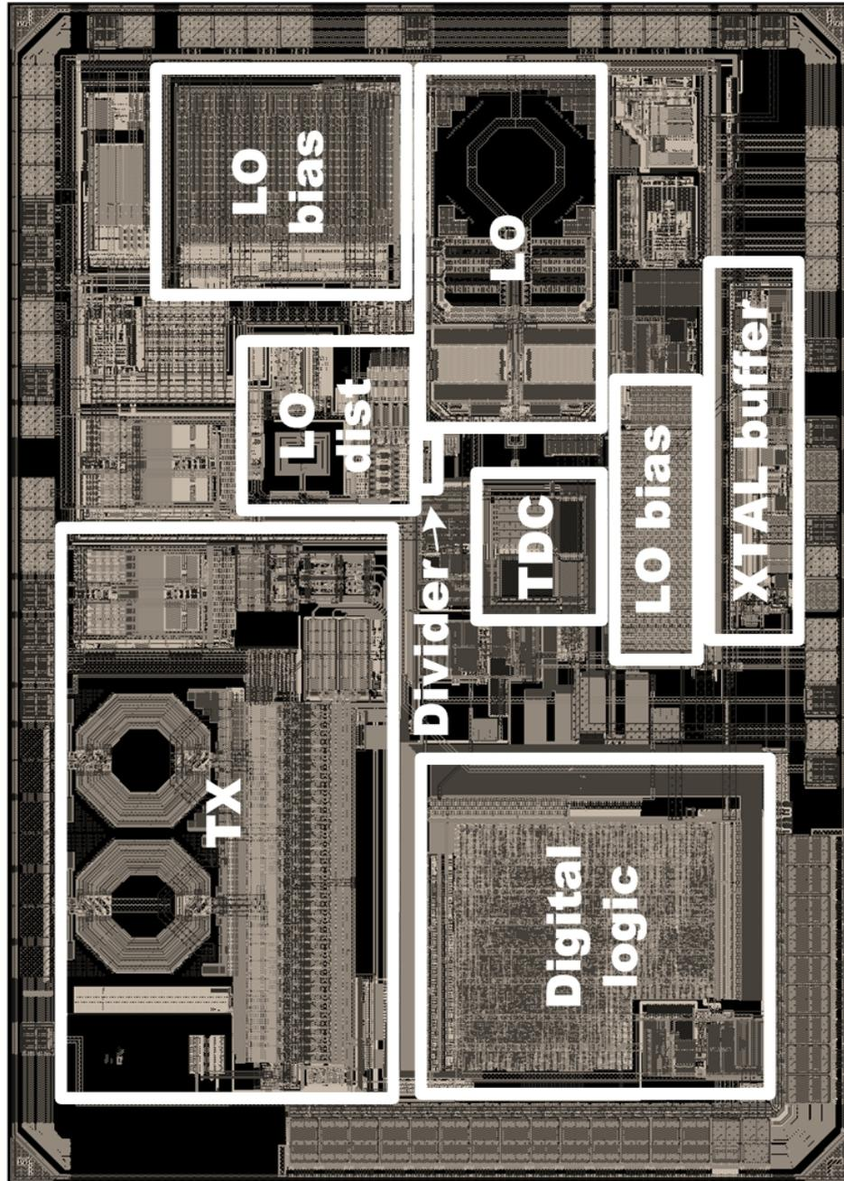
Figure 4.8: ADPLL prototype layout snapshot
