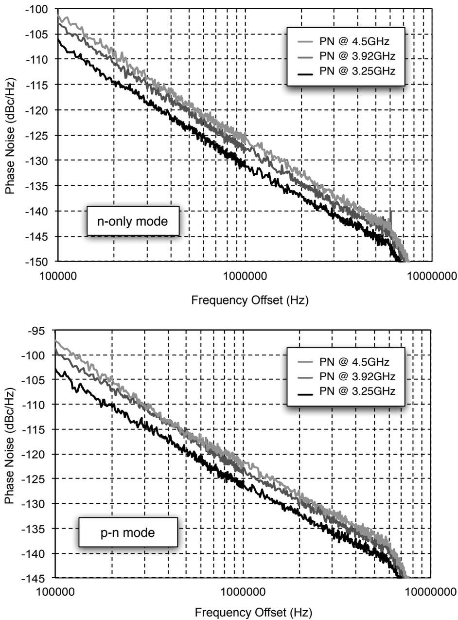
**Figure 4.18:** Phase noise measurements of the two DCO configurations at the minimum, center and maximum frequencies.
