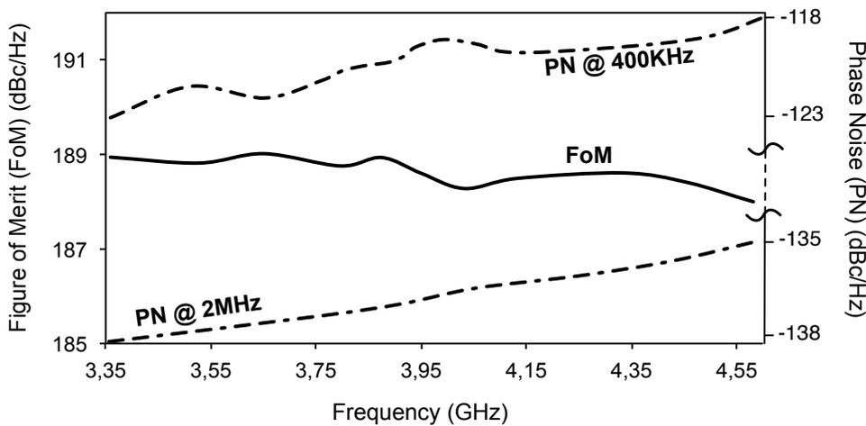
**Figure 4.21:** Phase noise measurements at the minimum, middle, and maximum oscillation frequency
