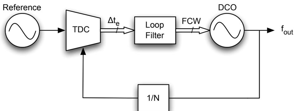
**Figure 1.1:** Diagram of an All Digital PLL.
