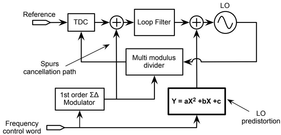
Figure 2.8: Predistortion calibration
