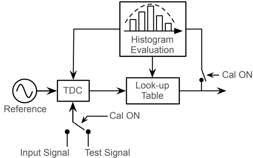
**Figure 2.5:** TDC linearity calibration loop
