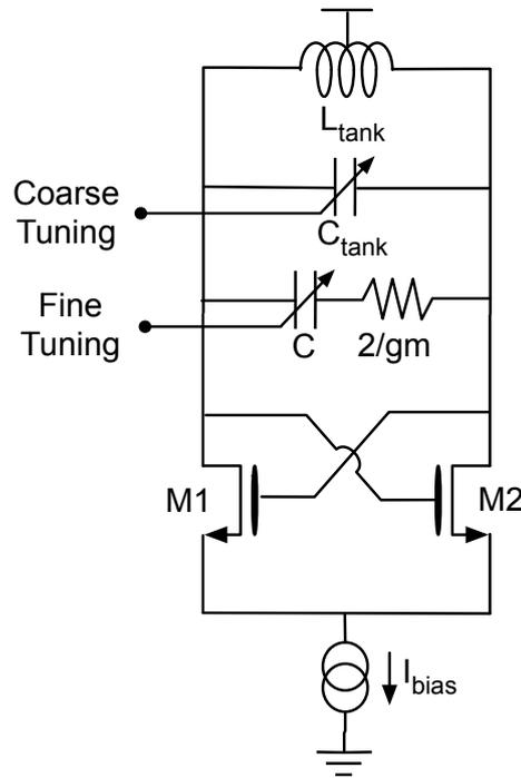
**Figure 1.17:** DCO scheme with the positive shrunk capacitance.
