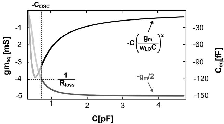
Figure 1.9: Real and Imaginary par of admittance  $Y$  ( $gm = 10mS$ ,  $R_{loss} = 250\Omega$ ,  $\omega_0 = 3.6GHz$ ).
