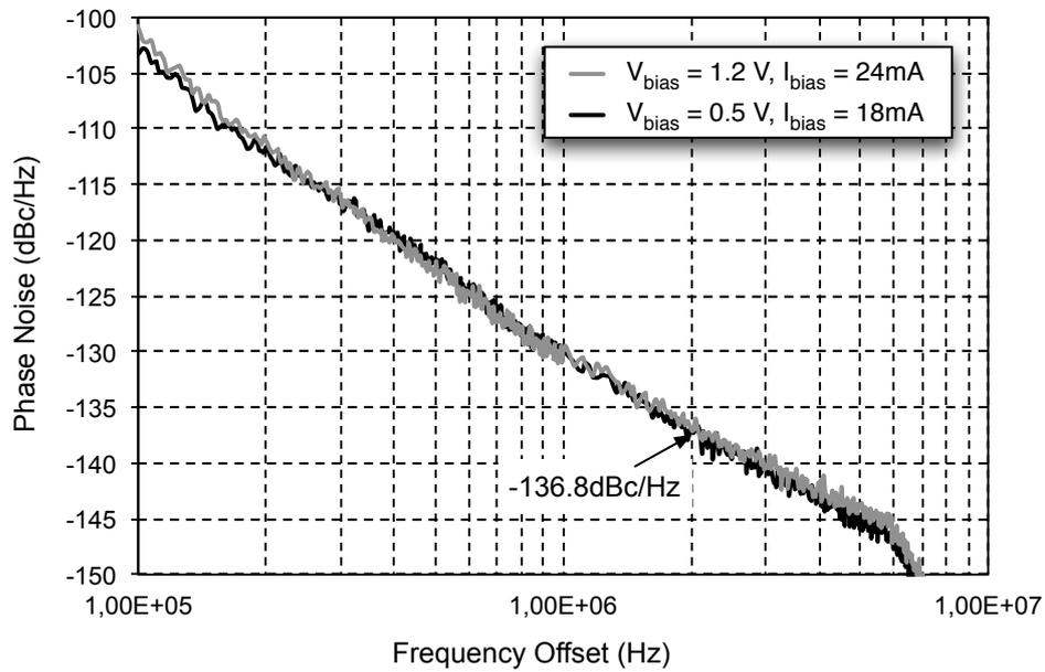
**Figure 4.23:** Phase noise plots at mid-band, for  $V_{bias} = 1.2\text{ V}$  and  $V_{bias} = 0.5\text{ V}$  with different current consumptions
