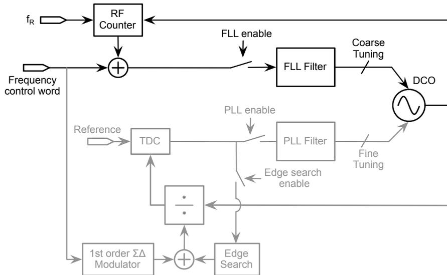
**Figure 2.10:** ADPLL frequency locked loop
