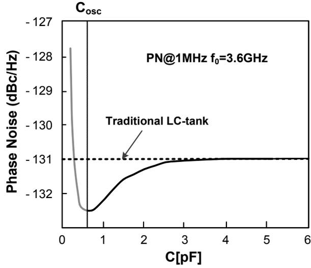
**Figure 1.15:** Phase noise versus degenerating capacitance  $C$ .
