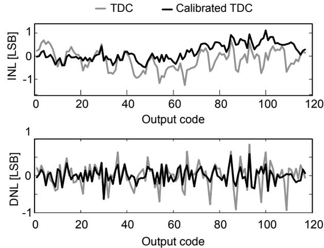
**Figure 4.12:** *Linearity measurements*
