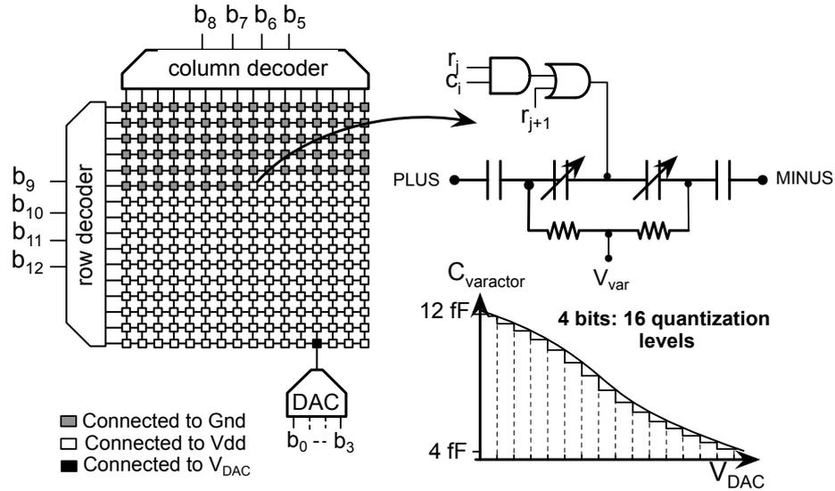
**Figure 2.7:** Fine-tuning bank of the ADPLL digitally controlled oscillator scheme
