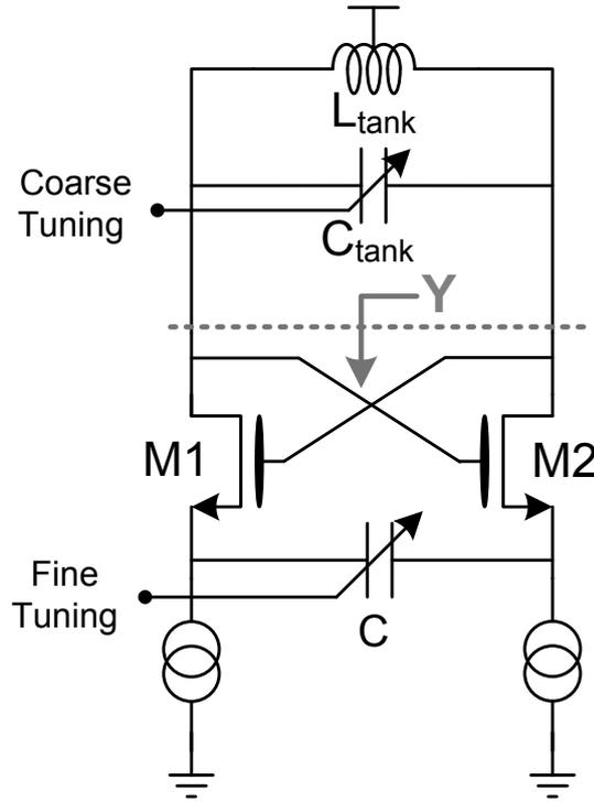
**Figure 1.7:** Capacitive Degeneration DCO scheme.
