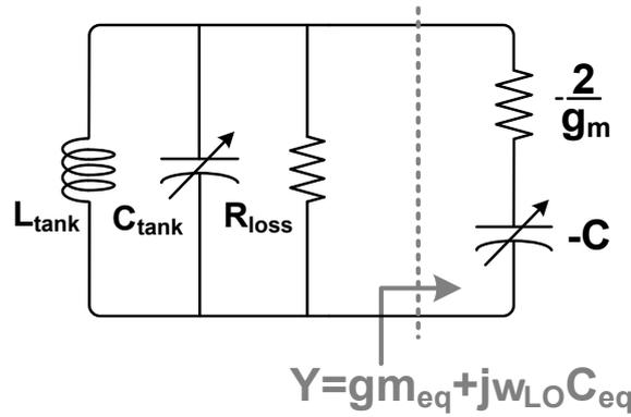
Figure 1.8: Capacitive Degeneration DCO equivalent scheme.
