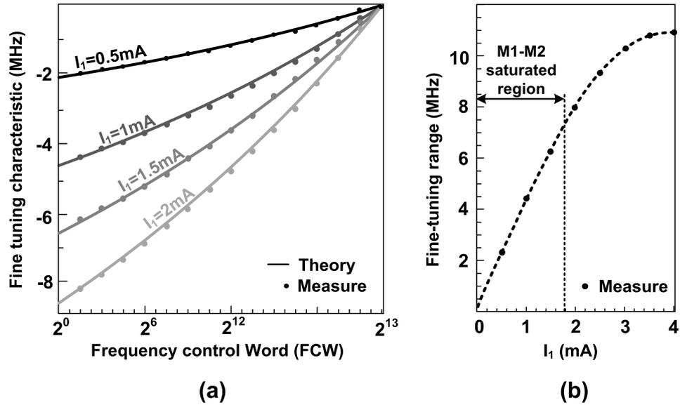
Figure 4.6: Fine-Tuning characteristic versus  $I_1$
