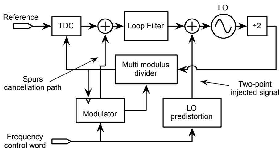
**Figure 2.1:** Fractional-N, two-points modulation ADPLL architecture.
