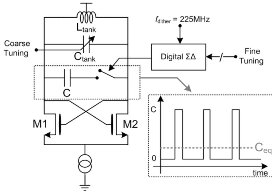
**Figure 1.5:** Scheme of the dithering technique.
