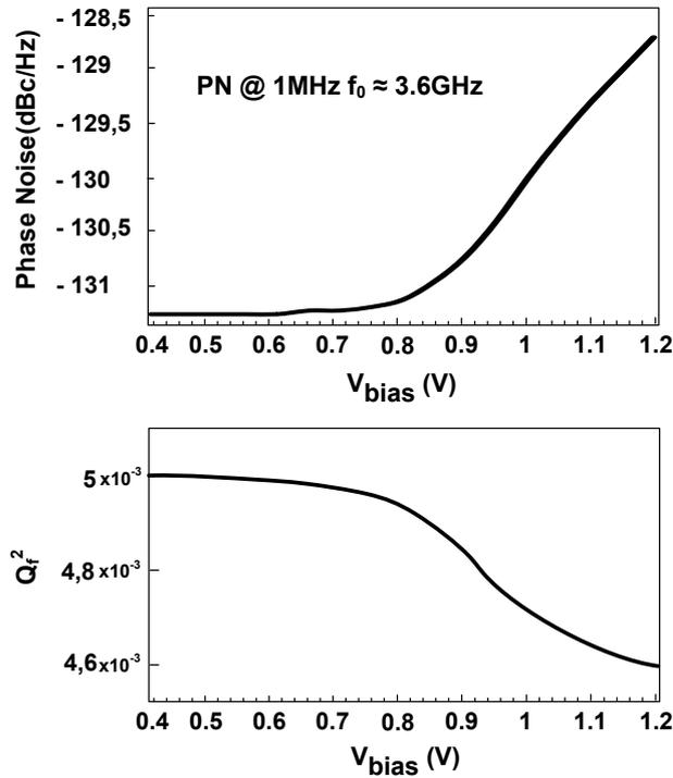
Figure 1.14: Phase noise and tuning range versus  $V_{bias}$ .
