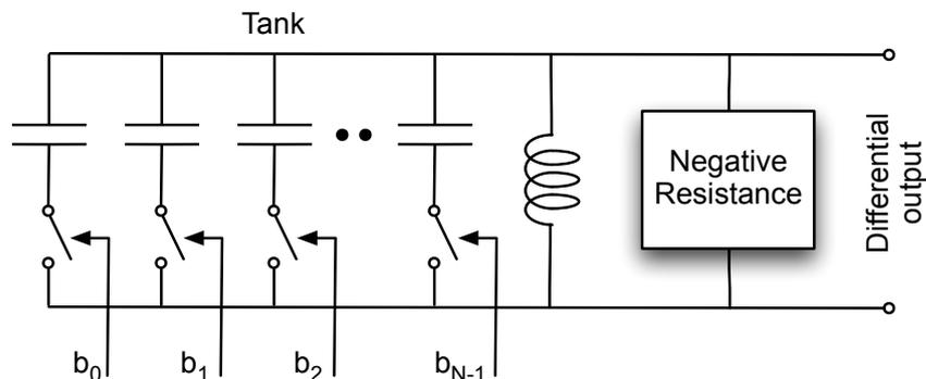
**Figure 1.3:** LC tank-based oscillator with switchable capacitors.
