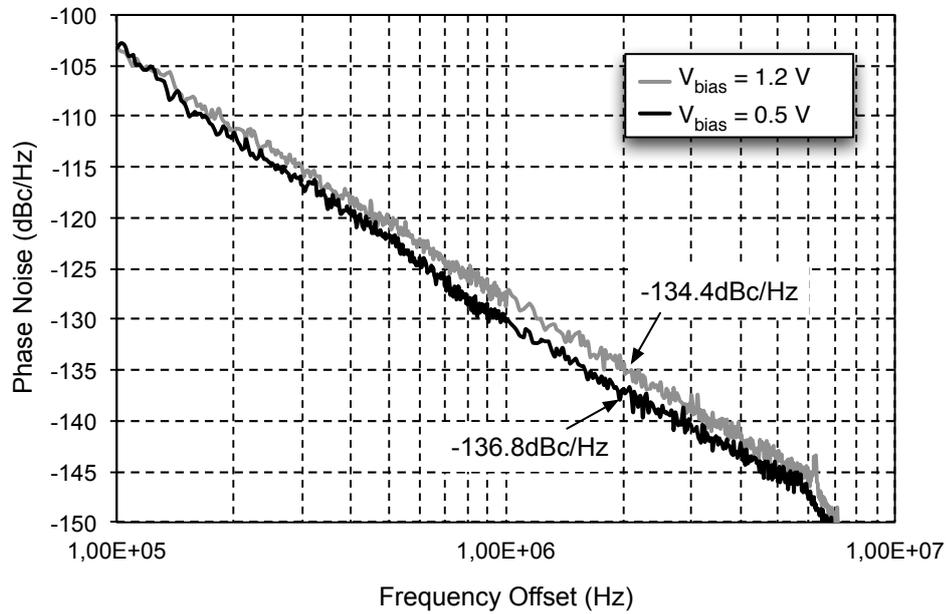
**Figure 4.22:** Phase noise measurements at mid-band, for  $V_{bias} = 1.2V$  ( $M_{C1}/M_{C2}$  operating in class-B), and  $V_{bias} = 0.5V$  ( $M_{C1}/M_{C2}$  operating in class-C), keeping a constant power consumption
