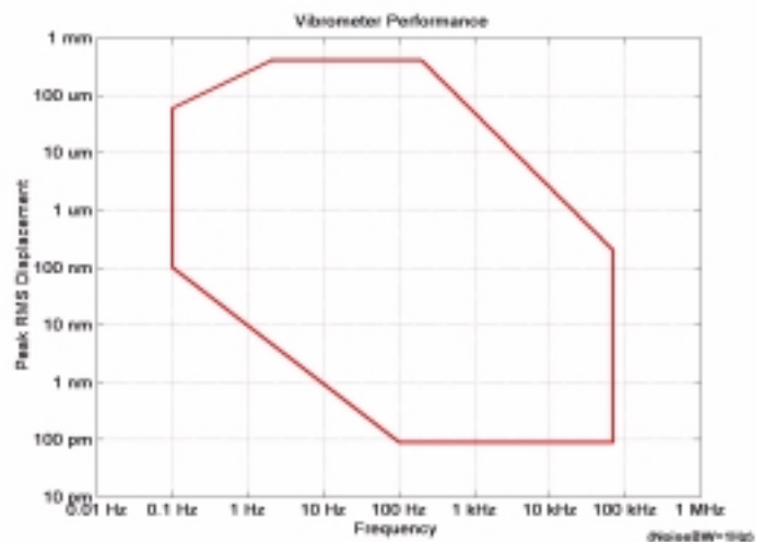
Fig.9. Nomogram reporting the vibrometer performance in the frequency-amplitude plane
