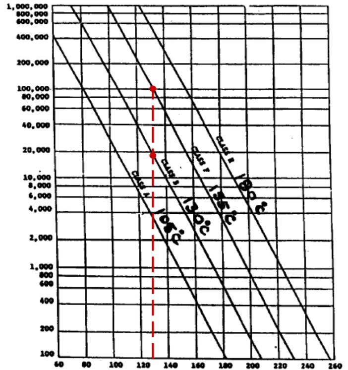
Fig. 1. Total winding temperature °C temperature versus life.
