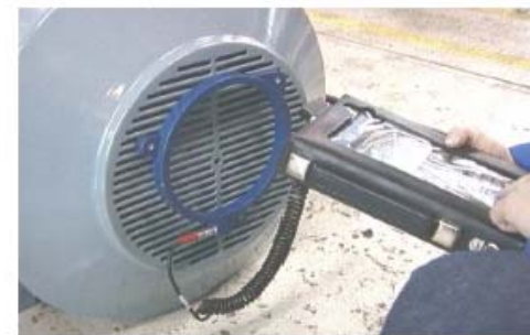
Axial flux measurement set up used in this thesis.
