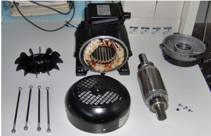
Three-phase induction motor of low power (2 kW), fed at low voltage (400 V), with aluminium die-cast rotor
