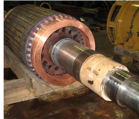
Fabricated cage rotor for a 3 MW motor, 6 kV, 2 poles
