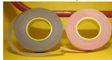
Figure 2: VPI and RR mica tape rolls
