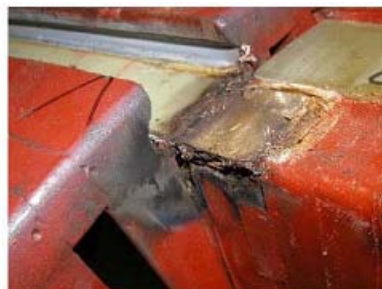
Fig. 13. Rotor top turn cracking caused an electrical ground fault from the rotor turn, through the ground insulation and to the rotor forging.
